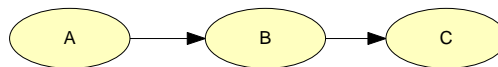
Figure A.1: An example of a Bayesian network with random variables, A , B , and C , each having two states.
